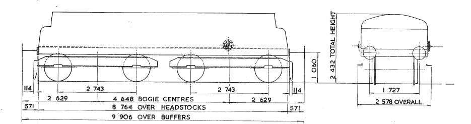
TARE - 36050 kg CARRYING CAPACITY-CAPACITY-MAX. SPEED - 60 mile/h WHEELS - 1105 DIA
