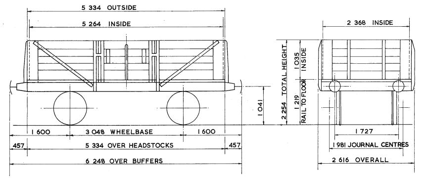
TARE -6<sup>450kg</sup> CARRYING CAPACITY- 13<sup>000kg</sup> CAPACITY- 12.827 m<sup>3</sup> MAX. SPEED - 45 mile/h
