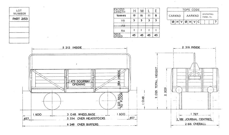
TARE - 6<sup>600 kg</sup> CARRYING CAPACITY - 13<sup>000 kg</sup> CAPACITY - 11. 885 m<sup>3</sup> MAX. SPEED - 45 mile/h WHEELS - 952 DIA. JOURNALS - 111 DIA. ROLLER BEARINGS
