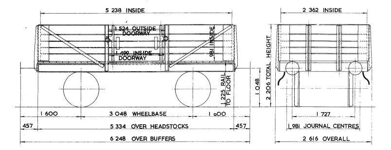
TARE – 6 <sup>400</sup> kg CARRYING CAPACITY – 13 <sup>000</sup> kg CAPACITY – 12. 162 m<sup>3</sup> MAX. SPEED – 45 mile/h
