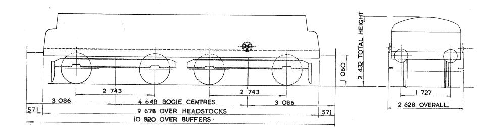
TARE - 36 050 kg CARRYING CAPACITY-CAPACITY-MAX. SPEED - 60 mile/h WHEELS - 1105 DIA. JOURNALS - 228 x 118 PLAIN BEARINGS
