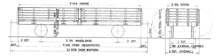
TARE - 10<sup>550 kg</sup> CARRYING CAPACITY - 20<sup>500 kg</sup> CAPACITY - 20. 317 m<sup>3</sup> MAX. SPEED - 50 mile/h WHEELS - 952 DIA. JOURNALS - 254 X 127 PLAIN BEARINGS
