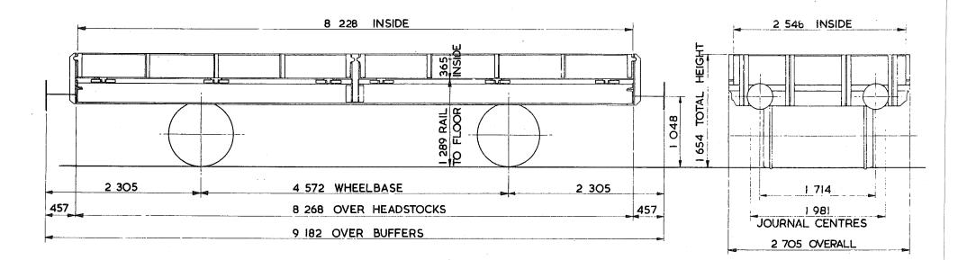
TARE - 9 800 kg CARRYING CAPACITY - 22500 kg CAPACITY --MAX. SPEED - 50 mile/h WHEELS - 952 DIA. JOURNALS - 254 x 127 PLAIN BEARINGS
