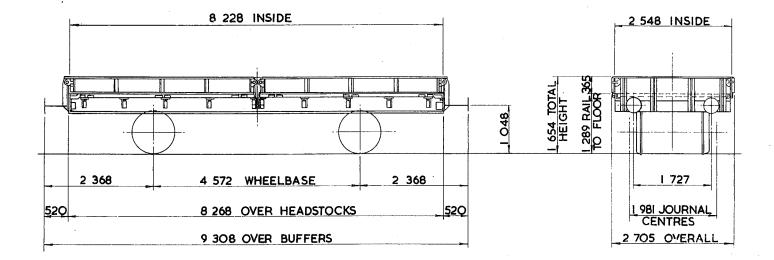
TARE – 9<sup>750 kg</sup> CARRYING CAPACITY-22<sup>500 kg</sup> CAPACITY-7.652 m<sup>3</sup>
