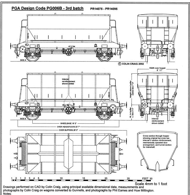
Built by Standard Wagon, Heywood in 1974. This batch was very similar to the 2nd batch of PG006B; the differences were: the headstocks were shallower, with no triangular step-down on the ends of the solebars, and the positioning of the brake air tank and distributor below the underframe.
