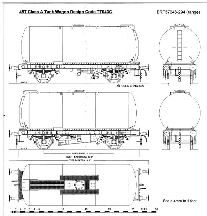
Drawing created in CAD by Colin Craig, based on the BR weight diagram dimensions, and web posted photographs.
