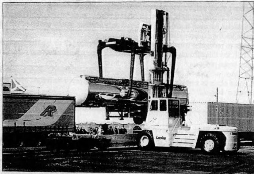
The first commercial 'Piggyback' services are due to start in June between Deanside, Glasgow and Willesden, London. During the official launch on May 15, the loading of lorry trailers onto 'Eurospine' wagons was demonstrated. The wagons can also carry standard containers, and one is already loaded on the right. HOWARD JOHNSTON.
