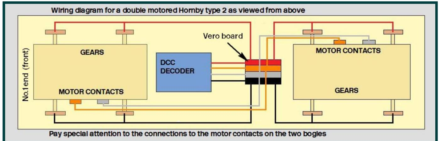
For DC operation all you need to do at this stage is link the red wires to orange and black to grey.
