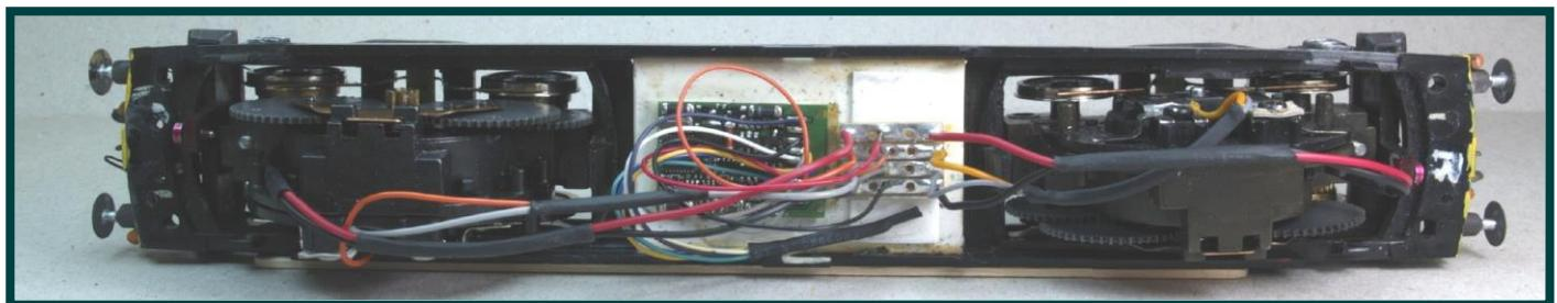
To protect your investment in the DCC decoder it is now important to check your wiring on a 'programming track'. Do not apply track power until you have confirmed that the DCC system will read the locomotive address.
