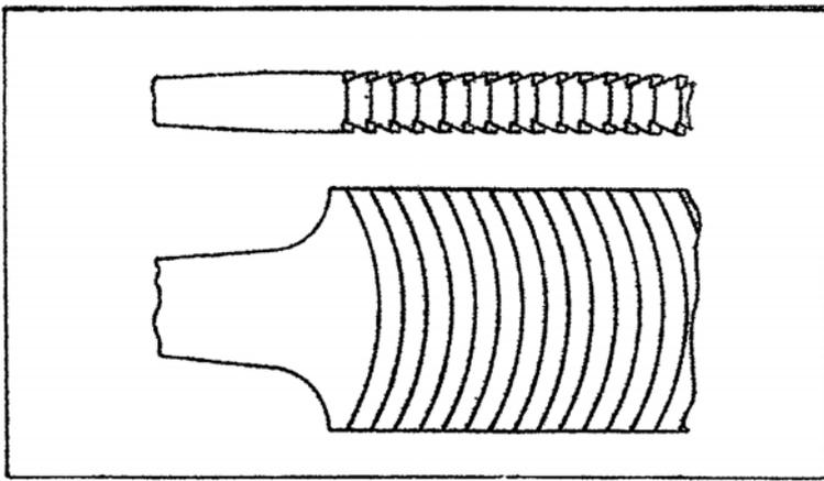
Most files are double cut, but it is often said that single cut gives a better finish on soft materials. Milling files, with single cut, curved, coarse, teeth, are very effective with materials like aluminium alloys and plastics.
